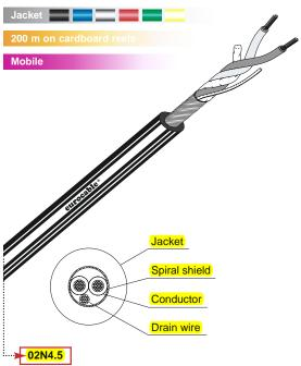
This cable which is 4,5 mm in diameter is suitable for Bantam patch cords. This extra flexible patch-cable is also ideal for situation where the space is critical.
